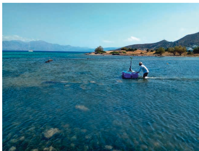
Figure 1. Acquisition of multi-frequency electromagnetic data at the archaeological site of Olous (Greece).
